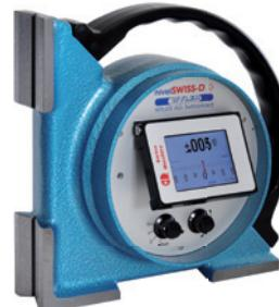
The measuring faces are carefully hand scraped to obtain an extraordinary precision. This makes the nivelsWISS-D extremely suitable for adjustments or checks on rectangular geometrical components of machine tools and structures. Both versions allow the direct connection to a laptop with a USB cable.
