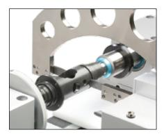
Diameter measurement in a groove
