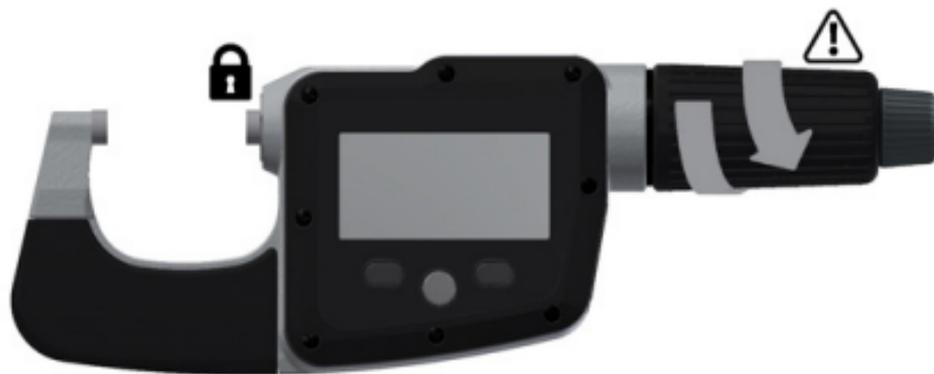
To unlock the spindle, rotate the speeder to disengage the lock, then keep rotating the controller to move the spindle forward.
