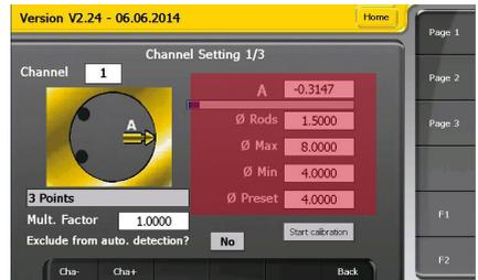
5. Insert the large ring on the instrument and click OK on the D300S
