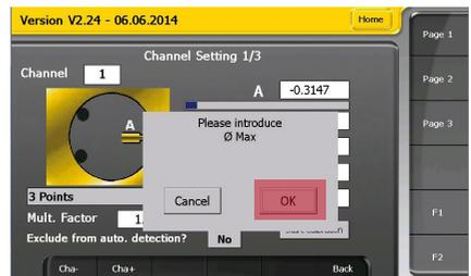
6. Insert the small ring on the instrument and click OK on the D300S
