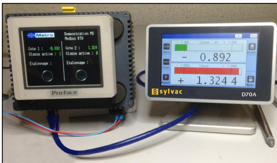
Example of a RTU Modbus communication with an automate Pro-face.
