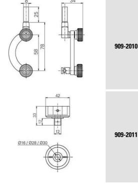
909-2010 Clamping device for test indicator
