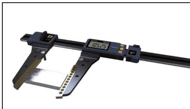
External measure with UL4
