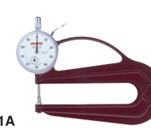
H-1A Graduation: 0.01mm Range: 0~10mm
