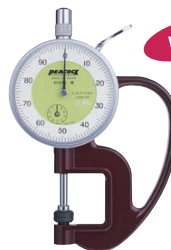
G-0.4N Graduation: 0.01mm Range: 0~10mm
