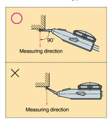
• In case they are not perpendicular, a correction by the following formula is necessary: Due to various measuring direction, the contact point sometimes can not be angled perpendicular to the measuring device.
